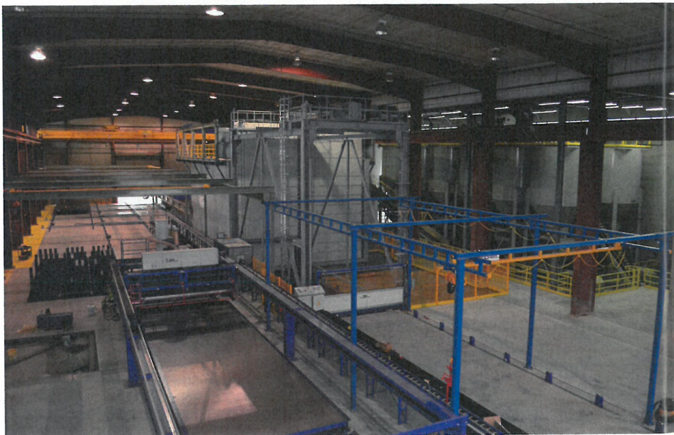
The plotting machine in the lower left corner inks a CAD file on to the pallet for precise alignment of shutters. Also shown is the curing chamber and rack operator in the middle and right hand side.
