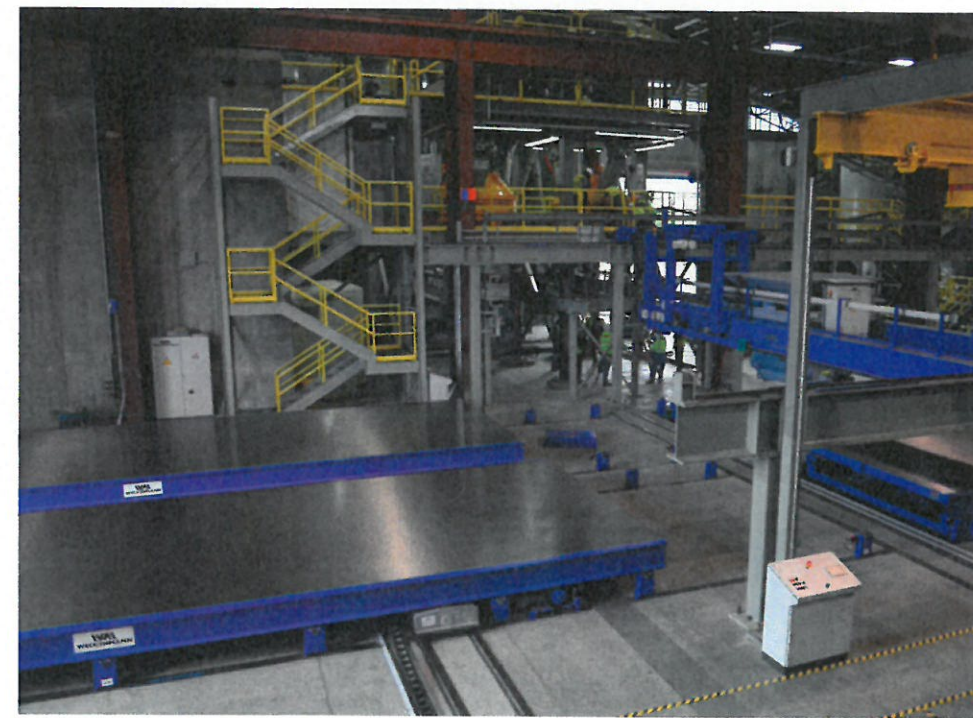
The batch station is ready to receive the pouring bucket (background) as two pallets are ready to enter the casting station (foreground).
