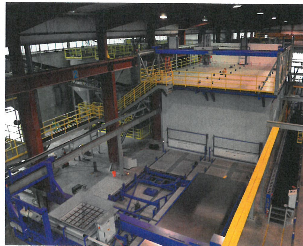
Overall view of the concrete placement stations. Two pouring buckets (one visible here) and a concrete spreader pour the concrete panels that will then move to the curing chamber by entering through the lower white doors. Directly above the chamber in the mezzanine is the troweling station where final finishes are applied to all products.
