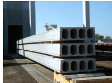
16" Hollow Core rolls out of Molin's plant
